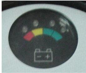
The remaining power indicated by the battery gauge will vary by the driving time incurred and how you ride. Repeated starting, stopping and climbing will consume power more quickly. The gauge is shown above.
