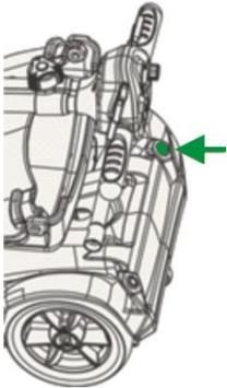
3. The green button (green arrow below) on the scooter should now be illuminated. Press it then release the button and the scooter will automatically unfold.
