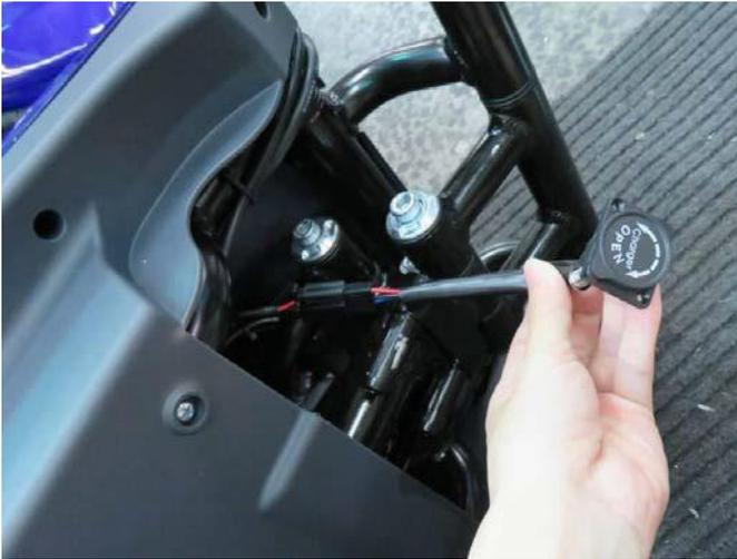
Install the cable, then proceed to charge the battery as described in the next section.
