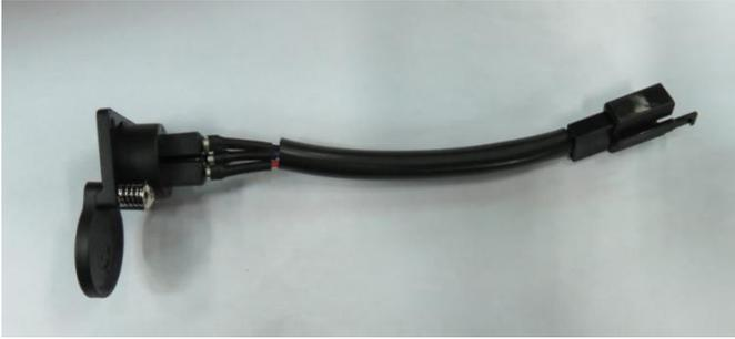
To install the charging cable, plug this in to connector cable at the front of the underside of the scooter (as shown below).
